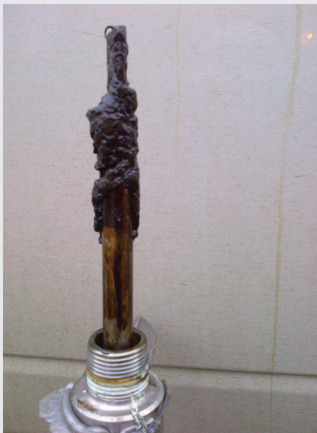
Sample of the organic deposits formed on a scale coupon installed at the heat exchanger.
